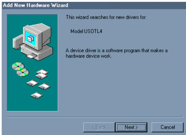
**#1.** Plug the USOTL4 into an available USB port on your computer or connected hub. The screen above appears, telling you that there is a new device plugged into the USB bus. Click on the **Next>** button.
