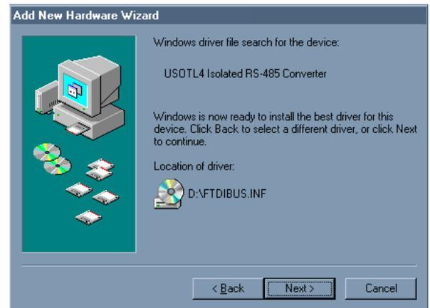
**#4.** The screen above appears. Make sure *Model USOTL4 (B&B's USB to Isolated RS-485)* is listed as the device. Then select the **Next>** button.
