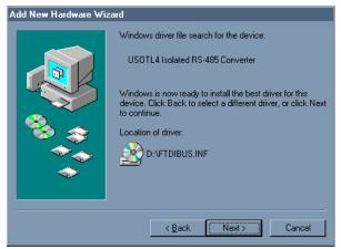
**#4.** The screen above appears. Make sure *Model USOTL4* (*B&B's USB to Isolated RS-485*) is listed as the device. Then select the **Next>** button.
