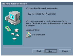
**#6.** You will also need to continue to install the serial port the same as installing the converter. Click the Next button followed by the Finish button. It will take a couple seconds for the serial port to be installed.
