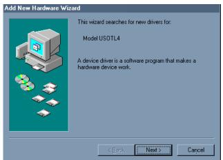
**#1.** Plug the USOTL4 into an available USB port on your computer or connected hub. The screen above appears, telling you that there is a new device plugged into the USB bus. Click on the **Next>** button.
