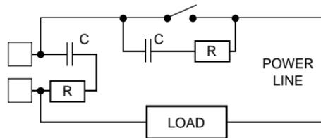
It is recommended to install an additional RC network across the external contacts as close to the instrument terminals as possible.
