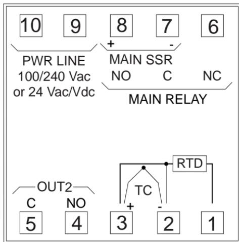
**NOTE:** When a relay output is used to drive an inductive load, connect an external snubber network (RC) across the terminals:
