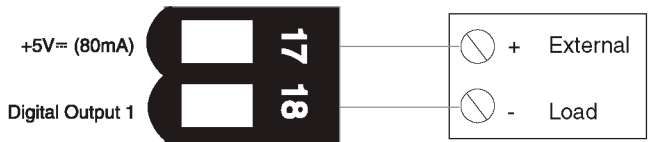
Figure 12.9c — Switched DC Example
